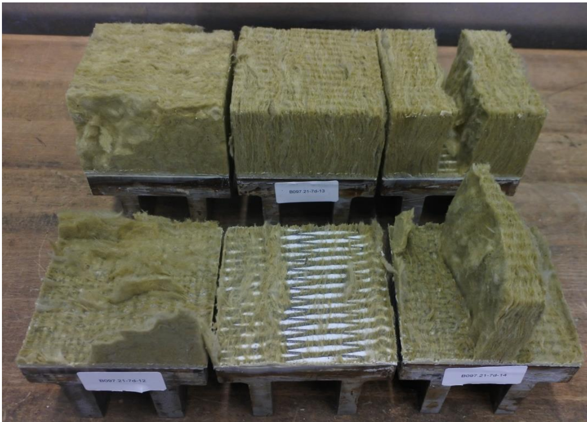
Figure 7: Failure figures of flatwise tensile test after 7 d of conditioning (DUR2); test series B097.21-7d-08...14, specimens -12...-14
