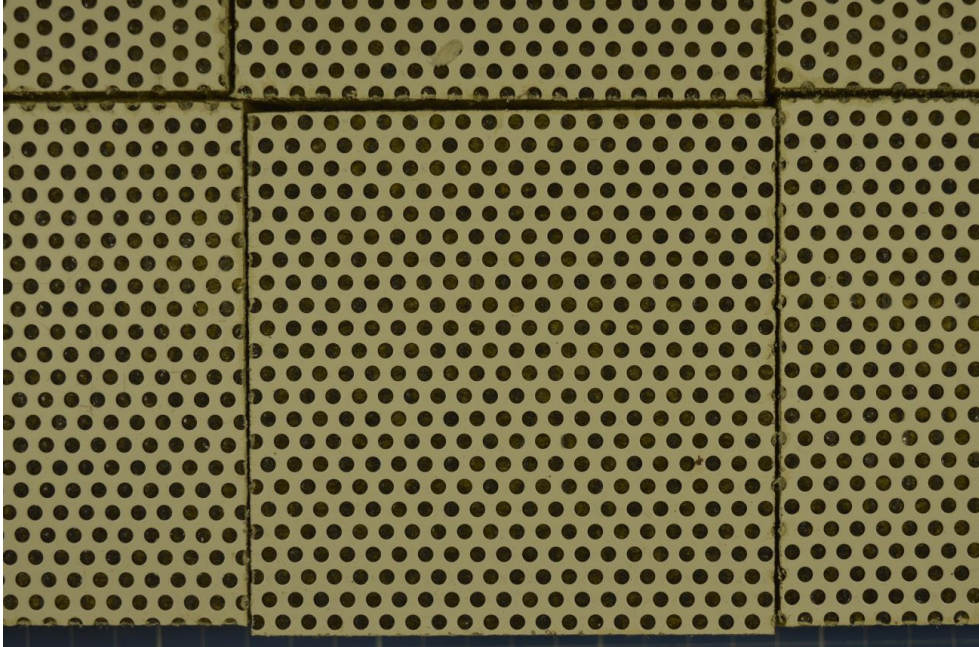
Figure 14: Perforated top layer after DUR2-conditioning (28 d), test series B097.21-28d-08...14
