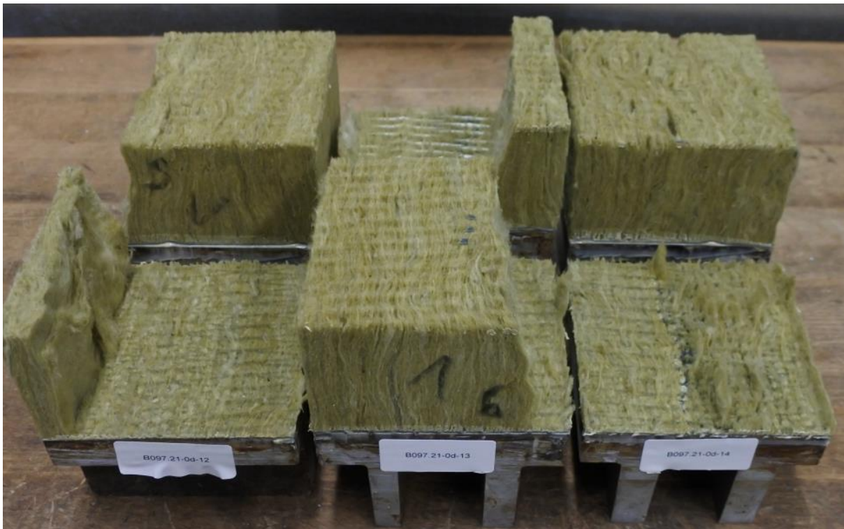
Figure 4: Failure figures of flatwise tensile test (reference without conditioning); test series B097.21-0d-08...14, specimens -12...-14
