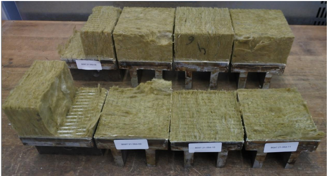
Figure 12: Failure figures of flatwise tensile test after 56 d of conditioning (DUR2); test series B097.21-56d-08...14, specimens -08...-11
