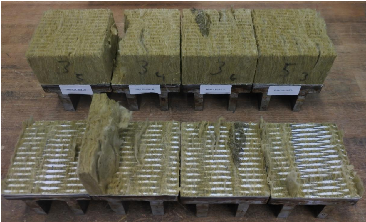
Figure 9: Failure figures of flatwise tensile test after 28 d of conditioning (DUR2); test series B097.21-28d-08...14, specimens -08...-11
