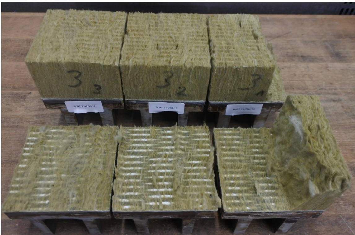
Figure 10: Failure figures of flatwise tensile test after 28 d of conditioning (DUR2); test series B097.21-28d-08...14, specimens -12...-14
