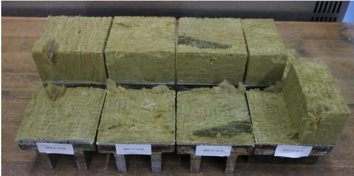
Figure 6: Failure figures of flatwise tensile test after 7 d conditioning (DUR2); test series B097.21-7d-08...14, specimens -08...-11
