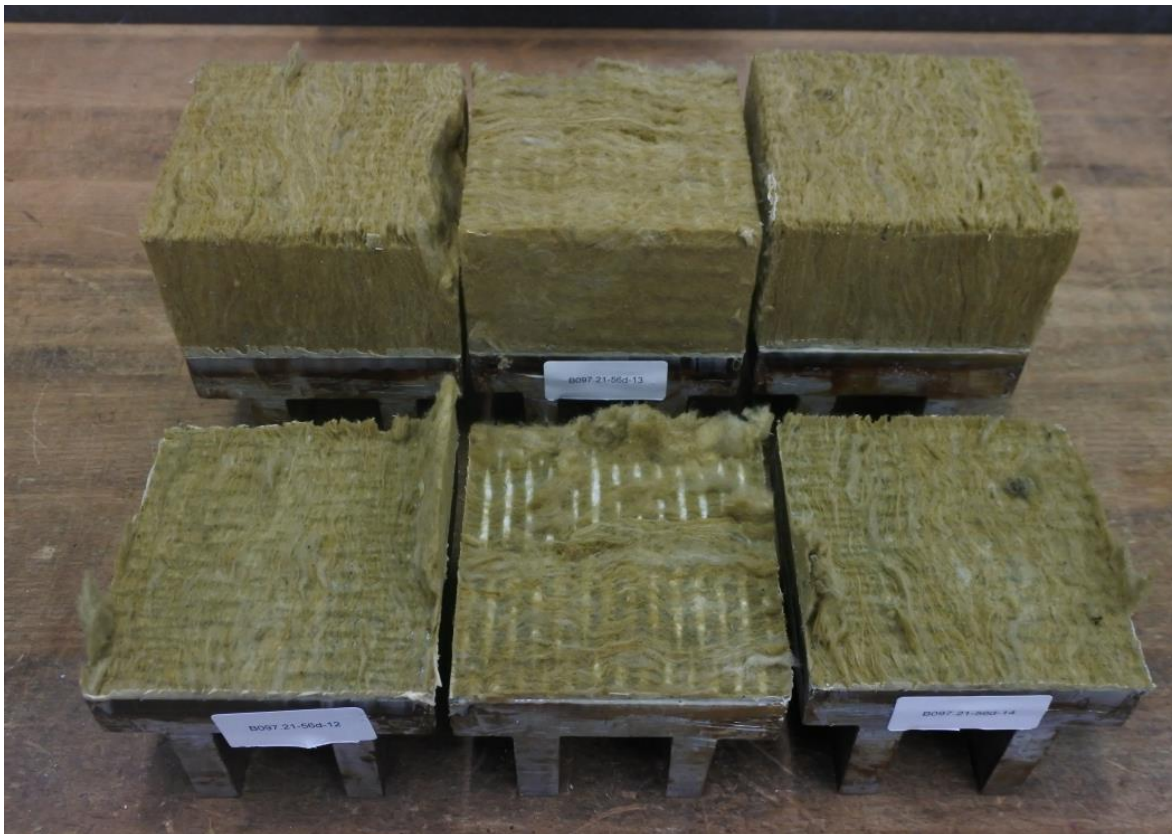
Figure 13: Failure figures of flatwise tensile test after 56 d of conditioning (DUR2); test series B097.21-56d-08...14, specimens -12...-14
